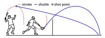
Fig. 10. Using *VirtualStroke* to select trajectories. The user sets a shot point and uses the controller as a racket to perform a stroke action. The target trajectories are selected based on the simulation of the stroke.
