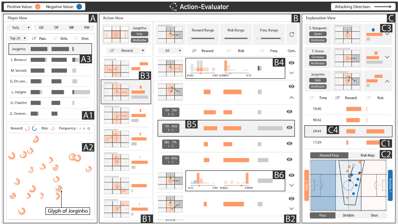
Fig. 4: System user interface. The interface contains three views: a player view (A), an action view (B), and an explanation view (C). The player view consists of a player ranking list (A1) to navigate players by importance and a player projection component (A2) to navigate players by similarity. The action view includes a match situation list (B1) to investigate action scores and an action score list (B2) to present those of different action choices. The adjustment view is composed of a record list (C1) and a ghost pitch (C2) to explain action scores to players.
